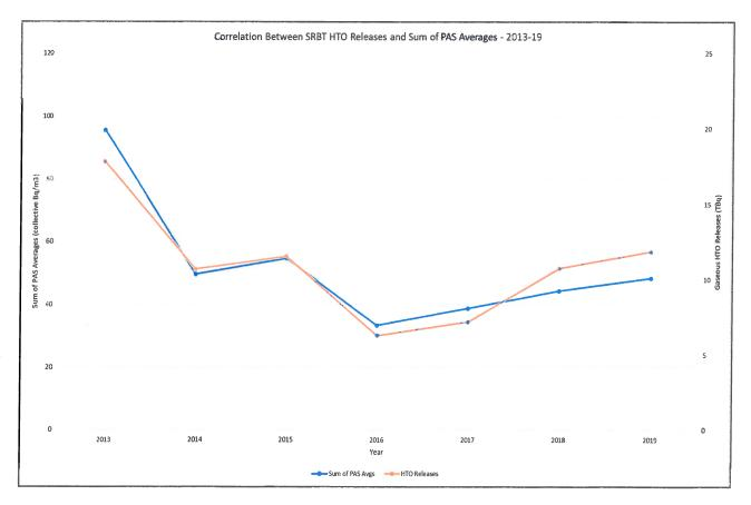
In 2019, the PAS concentrations trended slightly upwards in comparison to the previous three years. Likewise, emissions of tritium oxide were higher in 2019 and trended the same over that period. Similar relative trends are seen in each of the previous years of data.
